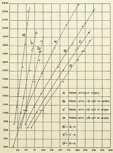
RESISTANCE OF WIRES AT GIVEN VELOCITIES
